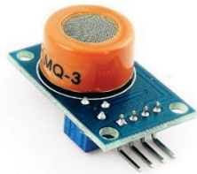
Фигура 10. Alcohol Ethanol Sensor Breath Gas Ethanol Detection MQ-3
